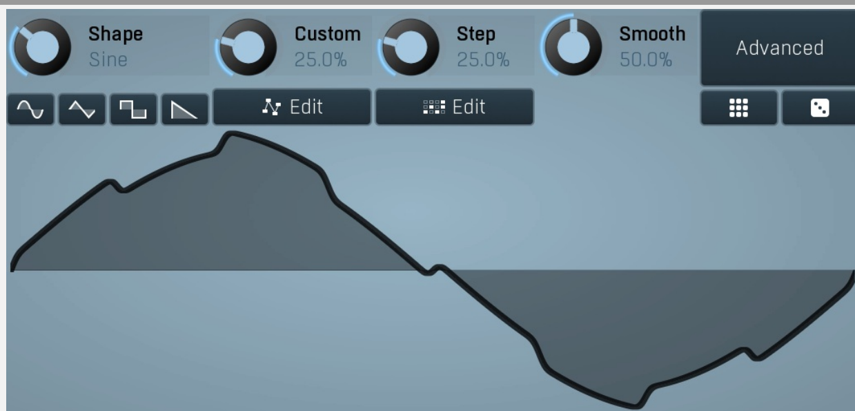
Signal generator in Normal mode works by generating the oscillator shape using a combination of several curves - a predefined set
