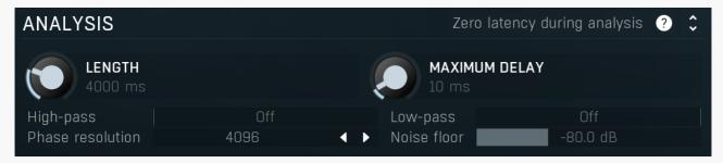
Analysis panel contains the parameters of the standard delay and phase inversion analysis.
