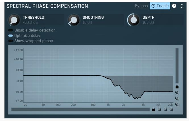
Spectral phase compensation panel contains parameters of the advanced algorithm, which directly adjusts the phase of all tracks to avoid phase cancellations. Please note that once you enable this panel, all of the instances in the group will start inducing latency.
