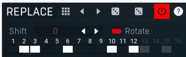
Replace panel controls the Replace operation. Replace operation replaces selected bits by the bits from the control signal. Control signal is a signal that is different from the input - it is used if the **delay** is used, **side-chain** is activated or **shift** is nonzero.
