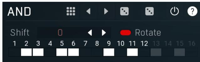
AND panel controls the AND operation. AND operation produces 1 if both inputs are 1. The processor operates differently if there is a control signal. Control signal is a signal that is different from the input - it is used if the **delay** is used, **side-chain** is activated or **shift** is nonzero.
