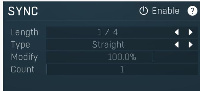
Synchronization panel contains parameters for the to-host synchronization.
