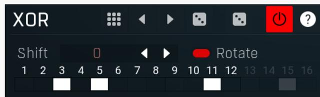
XOR panel controls the XOR operation. XOR operation produces 1 if both inputs are different. The processor operates differently if there is a control signal. Control signal is a signal that is different from the input - it is used if the **delay** is used, **side-chain** is activated or **shift** is nonzero.
