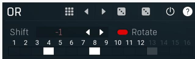
OR panel controls the OR operation. OR operation produces 1 if at least one of the inputs is 1. The processor operates differently if there is a control signal. Control signal is a signal that is different from the input - it is used if the **delay** is used, **side-chain** is activated or **shift** is nonzero.
