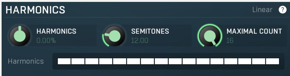
Harmonics panel contains parameters of the harmonics - clones of the main band created at higher frequencies derived from the frequency of the main band. This is often useful for removing natural noises, which usually bring some harmonics with them etc.
