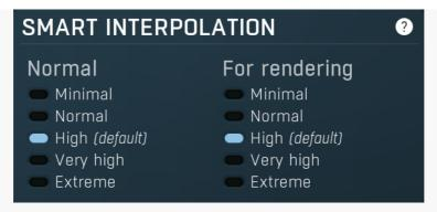
Smart interpolation panel controls the depth of the smart interpolation algorithm, which controls the parameters in order to provide maximum audio quality and lower the chance of zipper noise. Smart interpolation is engaged whenever you change any parameter via the GUI, modulators, multiparameters, MIDI or automation.
