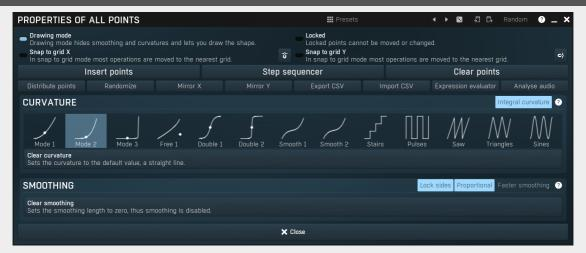
Envelope graph menu provides additional features which are used to edit the graph. Open the menu using right mouse button in the graph. Please note that if you select some points in the graph, or click on a point for example, the menu will be different and will cover only those features related to the selected set of points.
