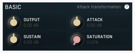
Basic panel contains the most important transient processor parameters.
