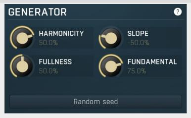
Generator panel contains parameters of the harmonics generator. By changing any of the parameters, the harmonics are changed, however only **Random seed** button changes the structure completely. The other parameters can be used to tweak the results.
