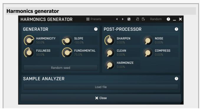
Harmonics generator is a powerful tool, that can generate various harmonics-based timbres and even analyze a sample file and extract harmonics from it.
