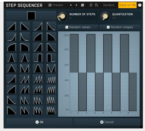
Signal generator step sequencer editor controls the step sequencer shape. You can have various numbers of steps each with a different value and shape. Note that for classic rectangular shapes the output can be very rough, hence it may be worth considering using **Smoothness** parameter to smooth out the resulting shape. This will use additional CPU power of course, but that should be negligible unless you modulate any of the signal generator parameters.
