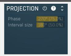
Projection panel contains parameters of projection onto the LFO oscillator shape, which takes the value generated by the modulator and puts it onto the LFO oscillator shape. This features is useful for several creative effects.
