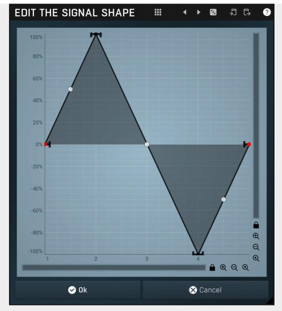
Signal generator custom shape editor controls the custom shape. You can edit virtually any shape that you can imagine and then blend it with the standard shapes, the step sequencer etc.
