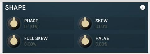
Shape panel contains parameters performing various transformations on the signal shape. Please note that most transformation require a significant amount of CPU resources, so you should not automate or modulate the signal shape if you are using them.
