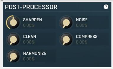
Post-processor panel contains parameters of the harmonics post-processor. The generator and sample analyzer first create a series of harmonics, the timbre. These harmonics are mixed depending on the **Sample ratio** parameter. After that the post-processor is engaged, which can further transform the harmonics in several ways.
