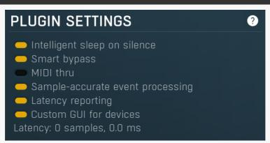
Plugin settings panel contains settings that control the behaviour of this plugin instance. These are properties that rarely need to be changed, so they have been moved here.
