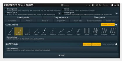
Envelope graph menu provides additional features which are used to edit the graph. Open the menu using right mouse button in the graph. Please note that if you select some points in the graph, or click on a point for example, the menu will be different and will cover only those features related to the selected set of points.
