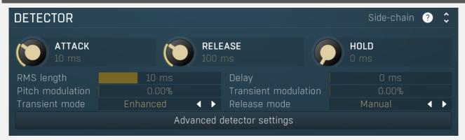
Detector panel contains the dynamic detector parameters, which control how the signal level is measured.
