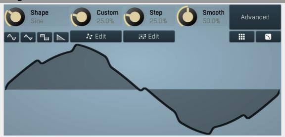
Signal generator in Normal mode works by generating the oscillator shape using a combination of several curves - a predefined set of standard curves, custom shape, step sequencer and custom sample. It also post-processes the shape using several filters including smoothing to custom transformations. This is especially useful when using the oscillator as an LFO (low-frequency-oscillator), where the harmonic contents does not really matter, but the shape does.
