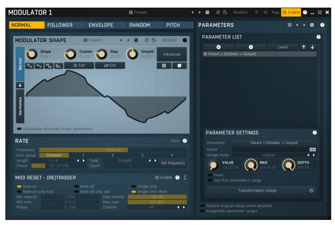
Modulator is an extremely advanced feature, which lets you change parameters automatically depending on various inputs. You can use this to add movement to your sound, respond to some plugins differently for louder sections, or even follow the pitch of the input.
