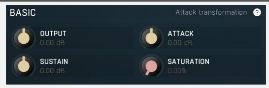
Basic panel contains the most important transient processor parameters.
