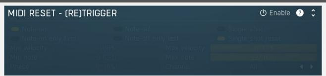
MIDI reset panel configures the MIDI reset feature, which will reset the oscillator when a MIDI note is received or its MIDI reset parameter is a target of another modulator or multiparameter. This way you can make the oscillator perform "in-sync" with your playing. Please note that once you enable it, the oscillator will not be in phase-sync with the host.
