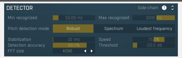
Detector panel contains parameters affecting the pitch detection. You can use them to make the detector work well with your audio material.
