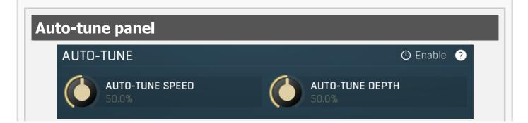
Auto-tune panel contains the automatic tuner parameters. When the pitch detector computes the pitch of the input signal, it can further adjust this value in the same way as an automatic tuner plugin, such as MAutoPitch, works. Note that there are no modifications to the input signal, only the pitch is detected differently.
