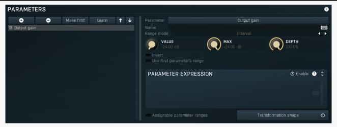
Parameters panel configures how the multiparameter assigns values to the target parameters.
