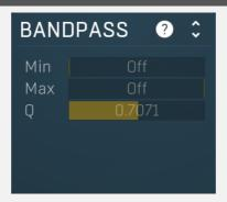
Band-pass panel contains parameters of the follower band-pass filter. Using this feature you can make the follower detect the level of just part of the spectrum instead of all frequencies. For example, when using band-pass from 20Hz to 100Hz the modulator will
