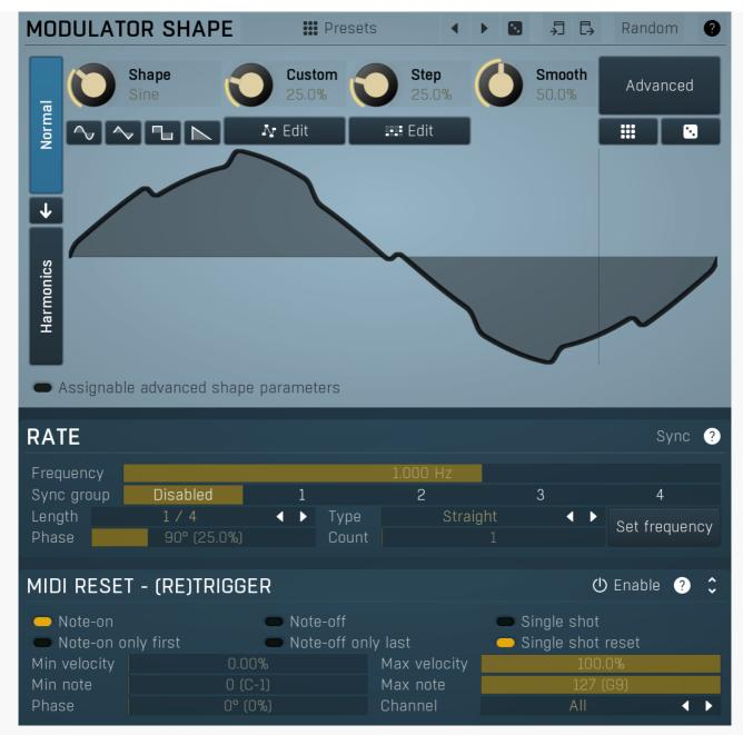
Normal mode makes the modulator work as a traditional low-frequency oscillator (LFO). Note that even if the modulator itself is running in a different mode, you can still blend this LFO using the **LFO modulation** parameter available on each tabbed page. The LFO parameters themselves are available on the first tabbed page only though.
