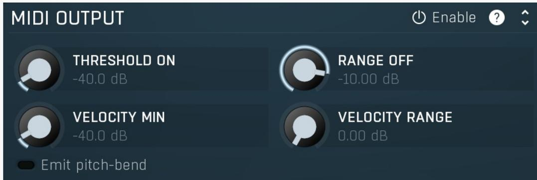
MIDI output panel contains parameters of the integrated audio->MIDI converter. You can use it by accessing the plugin's MIDI output. Please refer to your host's documentation for details about MIDI routing.
