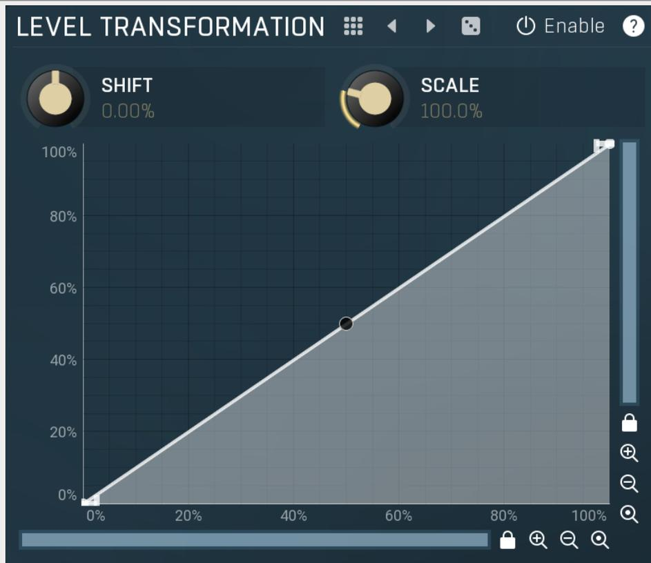
Level transformation graph lets you transform the dynamic gain according to the input level. The X axis contains the input level; the Y axis controls the output level, which is then used to set the dynamic gain.
