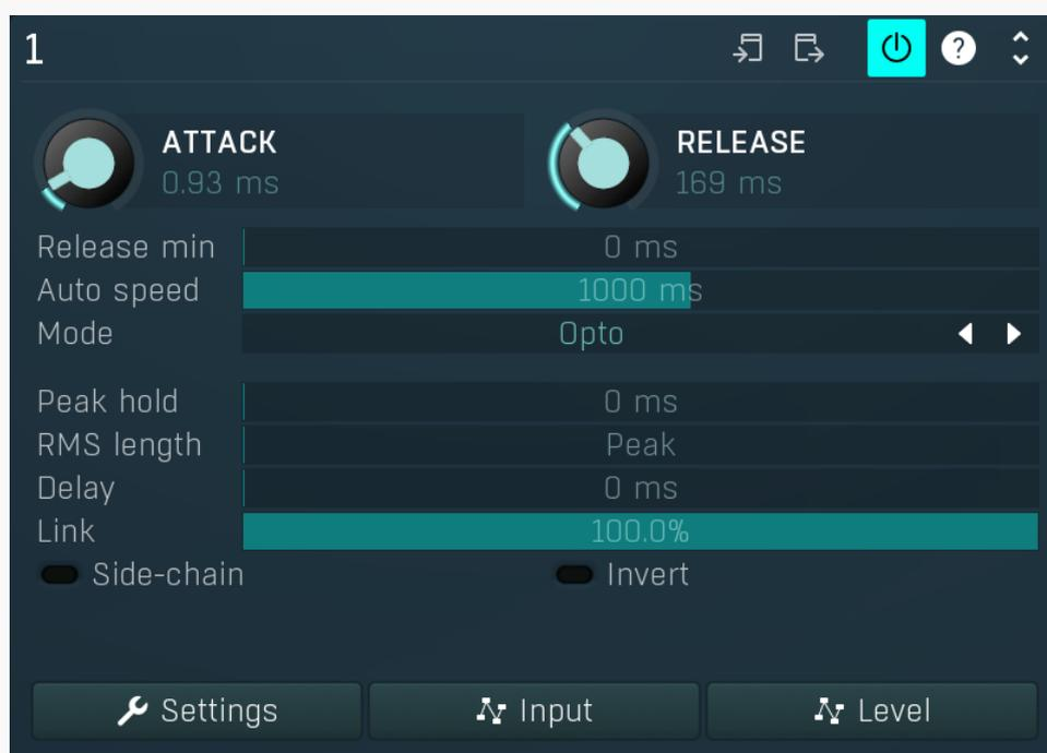
Follower panel contains the parameters defining how the plug-in determines the level of the source signal. Each follower operates on the original input or side-chain. Followers number 2 and higher provide additional features for combining their output with the current level generated by previous followers.
