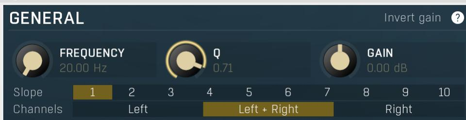
General panel contains standard filter settings such as frequency or Q. Most of these values are available directly from the band graph, but it may be necessary to use these controls for more accurate or textual access.
