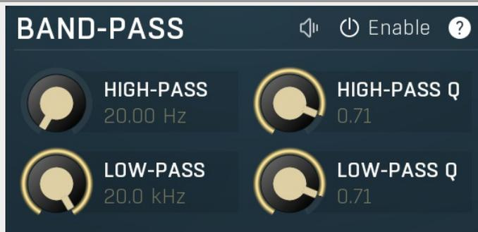
Band-pass panel contains parameters of the band pass, which you can use to process the signal that is used measure level of the band additionally. For example, you may want a band at high frequencies to react to bass content; you can do this by placing the band anywhere on the high frequencies and set the low-pass at say 200Hz.
