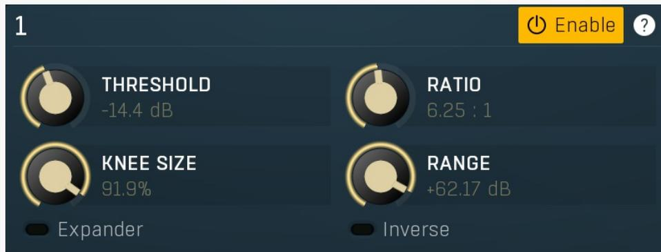
Processor panel contains parameters of the processor, which defines one segment in the transfer curve. It can behave like a compressor or expander.
