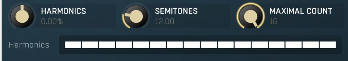
Harmonics panel contains parameters of the harmonics - clones of the main band created at higher frequencies derived from the frequency of the main band. This is often useful for removing natural noises, which usually bring some harmonics with them etc.
