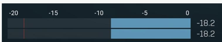
Meters display gain-reduction for each channel being processed. Also it contains controls to manipulate time-graphs shown in the transformation shape graph above.
