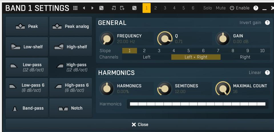
Band settings window contains settings for the particular band and can be displayed by right-clicking on a band or from a band list (if provided). On the left side you can see list of available filters, click on one to select it. On the right side, additional options and features are available.
