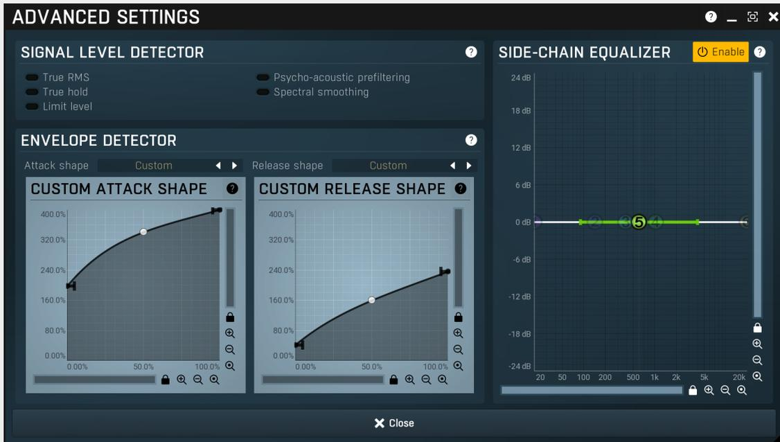
Advanced settings contains more esoteric and advanced settings of the level detector. These include various kinds of detector signal preprocessing, attack & release responses and custom shapes, etc.
